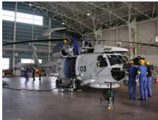
(SH-60K整備作業)
