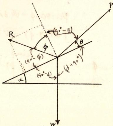
$$\left. \begin{aligned} W \sin \alpha &= F \\ W \cos \alpha &= N \end{aligned} \right\} \frac{F}{N} = \mu \quad \mu = \tan \alpha = \tan \phi$$
