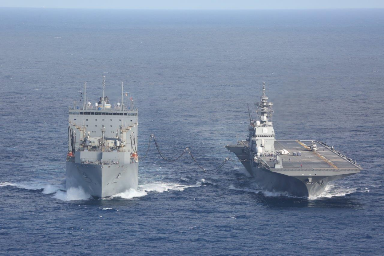
JS KAGA (right) conducted Replenishment at Sea with USNS WASHINGTON CHAMBERS (left)
