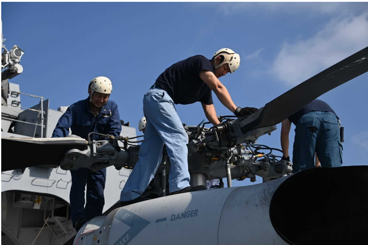
JS "AKEBONO" crew members conducting maintenance of a ship-board helicopter
