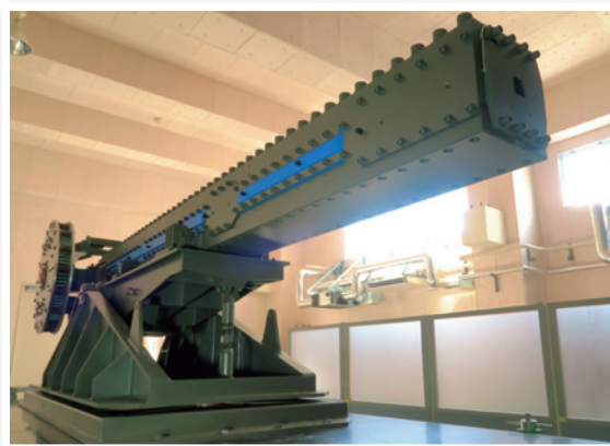
Railgun (electromagnetic gun) under research at the Acquisition, Technology & Logistics Agency
