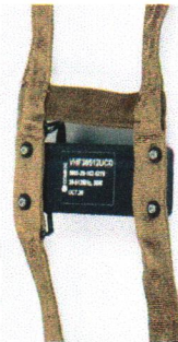
Centre junction of antenna
