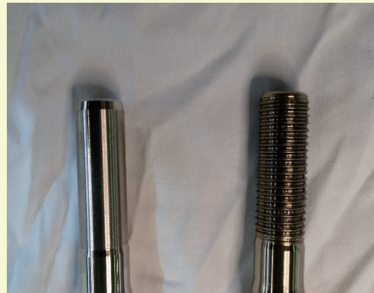
Before (left) and after (right) thread rolling
