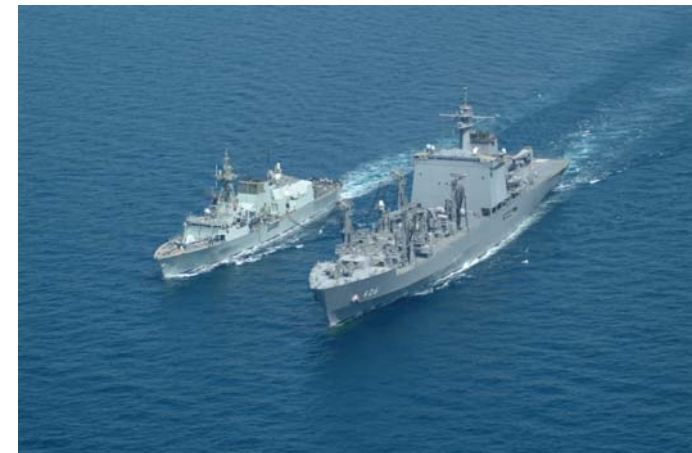
( Oiler "Oumi" replenishing fuel to Canadian frigate)
