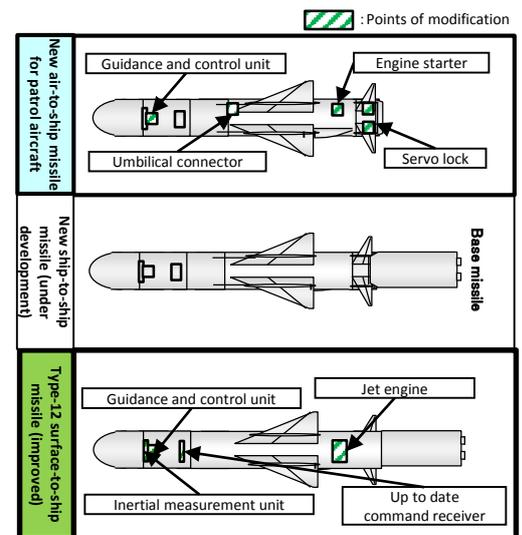
*Image of the standardization of the Type 12 surface-to-ship missile (improved) and a new air-to-ship missile for patrol aircraft*
