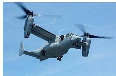
Tilt-rotor aircraft (V-22)
