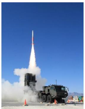
Type-03 middle-range surface-to-air missile (modified) (prototype)
