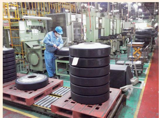
Deburring work for track rollers after rubber bonding, and finished products
