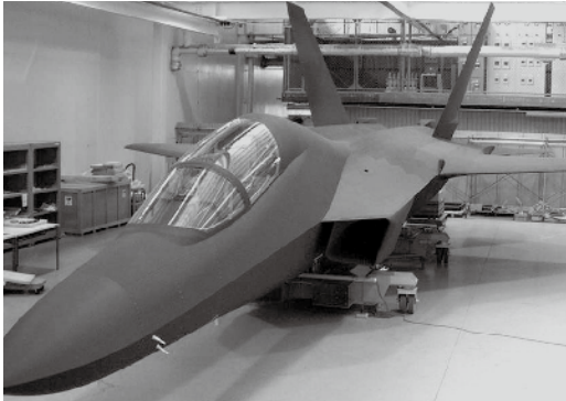
An actual-size model of the high maneuverability and stealth aircraft currently being researched at the Technical Research & Development Institute
