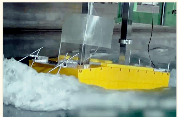
船舶水槽での水陸両用車模型試験 Tank Test for Performance of Amphibious Vehicle
