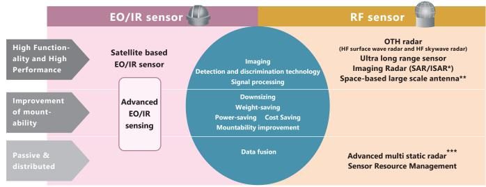
\* SAR utilizes the flight path of the platform and ISAR utilizes the motion of the target to form a large virtual aperture and generate high resolution images. \*\* GEO-based km-scale power transmission antenna technology to be used by the Space Solar Power System (SSPS).
