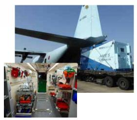
Aeromedical Evacuation Unit Type 2 is a container used to evacuate seriously ill or injured individuals and can be mounted on a C-130H or C-2 transportation aircraft. Once medical equipment and materials are installed within the unit. it has advanced medical monitoring and paramedic capabilities on par with an ICU.
