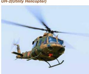
With improved performance and safety features, the UH-2 provides high capability while maintaining its long-established reputation for utility and reliability. The aircraft is a combination of the basic fuselage proven over numerous years of military operations and the newest dynamic components and avionics available today.
