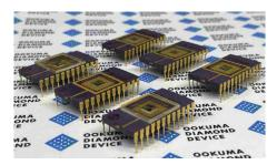
The world's first diamond semiconductor amplifier circuit has successfully demonstrated reliable operation under high temperature, specifically for a week at 300°C. This achievement marks a significant milestone towards the practical application of diamond semiconductor devices.
