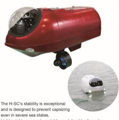
Lightweight, compact, portable, and durable, it can be transported to distant seas, launched from ships, and dropped in the air. Autonomous control and automatic selection of multiple communication methods make this USV robust and highly maneuverable.
