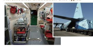
Aeromedical Evacuation Unit Type 2 is a container used to evacuate seriously ill or injured individuals and can be mounted on a C-130H or C-2 transportation aircraft. Once medical equipment and materials are installed within the unit, it has advanced medical monitoring and paramedic capabilities on par with an ICU.
