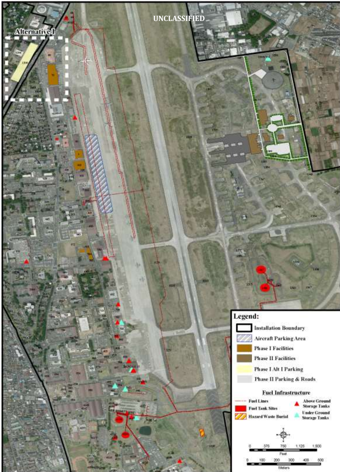
(U) Figure 3-7. Fuel Storage and Infrastructure
