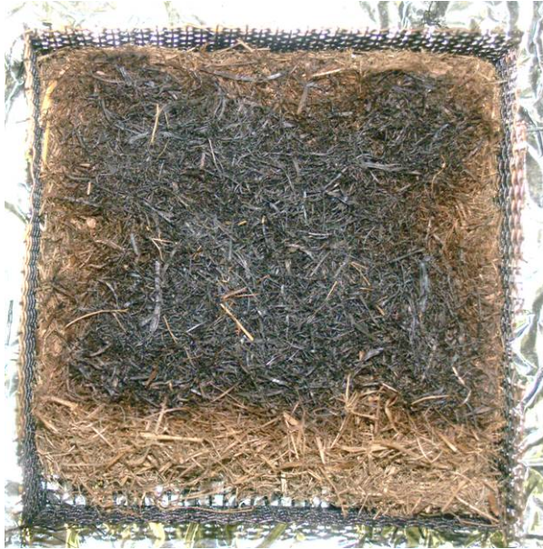
Figure 58. Bottom (left) and top (right) views of a fine Florida grass fuel bed are shown after the fuel was removed from the heated plate held at 310 °C with no wind applied. Glowing combustion was not observed.
