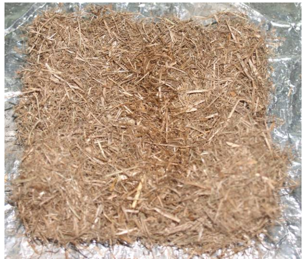
Figure 59. Bottom (left) and top (right) views of a fine Florida grass fuel bed are shown after the fuel was removed from the heated plate held at 290 °C with a low wind applied. Glowing combustion was not observed.
