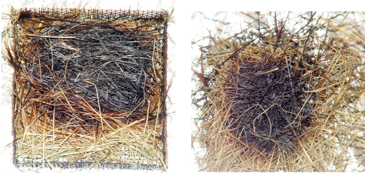
Figure 36. Bottom (left) and top (right) views of a May tall fescue fuel bed are shown after the fuel was removed from the heated plate held at 311 °C with no wind applied. Glowing combustion was not observed.
