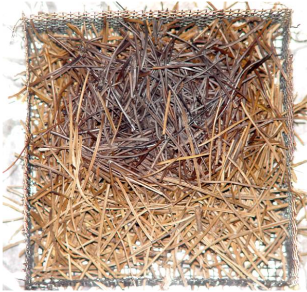
Figure 61. Bottom (left) and top (right) views of a pine needle fuel bed are shown after the fuel was removed from the heated plate held at 290 °C with no wind applied. No glowing combustion was observed.
