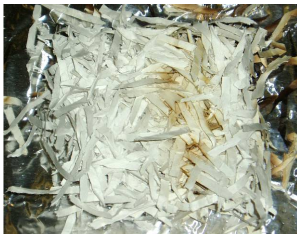
Figure 25. Bottom (left) and top (right) views of a shredded newsprint fuel bed are shown after the fuel was removed from the heated plate held at 333 °C with a low wind applied. Glowing combustion was not observed.
