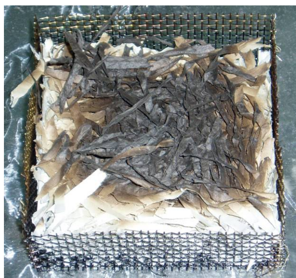
Figure 26. Bottom (left) and top (right) views of a shredded newsprint fuel bed are shown after the fuel was removed from the heated plate held at 332 °C with no wind applied. Glowing combustion was not observed.
