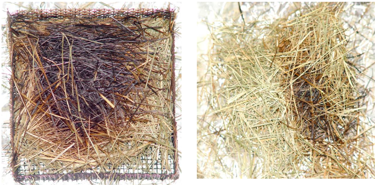
Figure 37. Bottom (left) and top (right) views of a May tall fescue fuel bed are shown after the fuel was removed from the heated plate held at 311 °C with a low wind applied. Glowing combustion was not observed.
