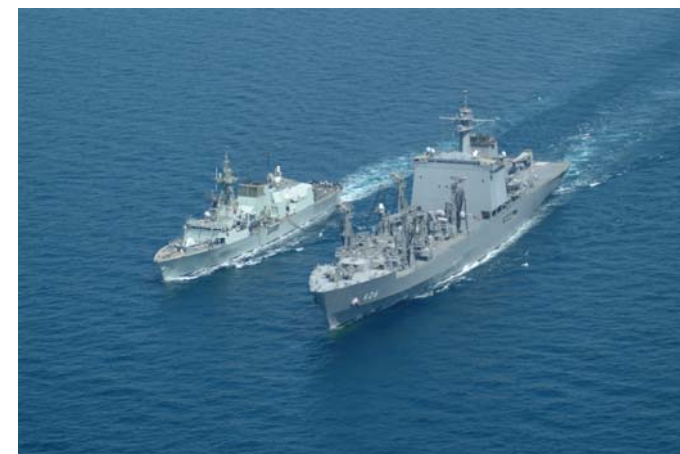
( Oiler "Oumi" replenishing fuel to Canadian frigate)
