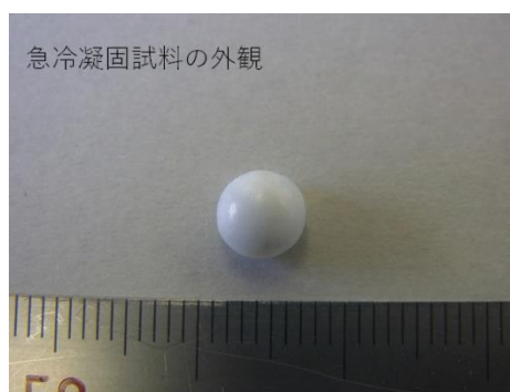
図 85 \text{LaAl}_{11}\text{O}_{18}/\text{LaAlO}_3/\text{La}_2\text{Hf}_2\text{O}_7 共晶の as-melt 材外観
