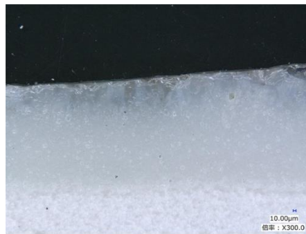
図 139 \text{LaAl}_{11}\text{O}_{18}/\text{La}_2\text{Hf}_2\text{O}_7/\text{LaAlO}_3 共晶皮膜断面(1300°C)
