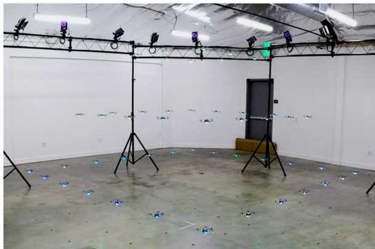
Fig. 5. Forty-nine Crazyflies flying in a 4-layer rotating pyramid formation. The bottom layer is 3 m x 3 m with 0.5 m spacing between vehicles.
