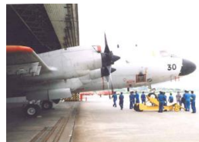
P-3C aircraft spending hours to tow into the hanger with its nose landing gear lifted.
