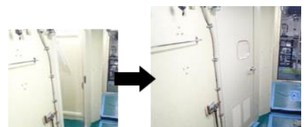
Development of Women's Quarters (Installation of corridor doors in front of shower rooms on naval vessels)
