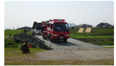
Type-07 mobility support bridge (disaster management exercise on passage of fire engines)
