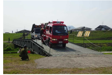
Type-07 mobility support bridge (disaster management exercise on passage of fire engines)
